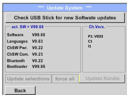
If after pressing the button “*Check USB Stick for new Software updates*” the following messages appear in the window, the LD 500 is not properly connected to the USB flash drive or there are no files available.
