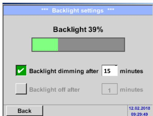
With the help of the *Backlight dimming after* button, after a definable time interval (here after 15 minutes), the *Backlight* can be reduced to the minimum.
