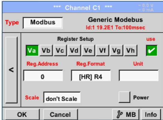
The measurement values are kept in the registers of the sensor and can be addressed via Modbus and read by the PI 500
