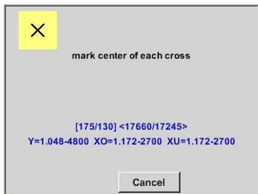
If necessary, the touch-screen calibration can be changed here.
