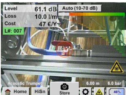
After switching on the LD 500, the initialization takes place and then switch to leakage display
