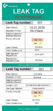
If necessary, fill out the Leak Tag-form and attach it to the measuring location.
