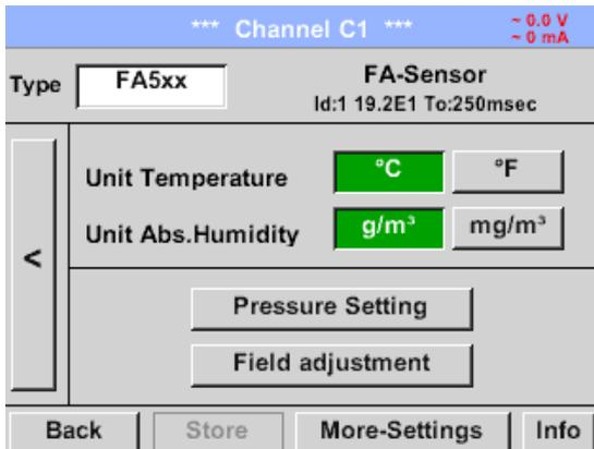
Unit selection for temperature and humidity by pressing the button °C, °F,  $g/m^3$  or  $mg/m^3$ .
