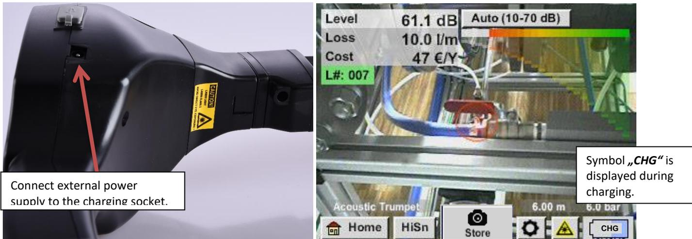
The LD 500 checks the charging status of the battery and starts the charging process automatically if necessary.
