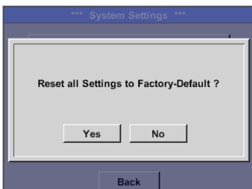
Bevor the settings are changed to the production default settings a safety prompt is displayed and must be confirmed by pressing the button „Yes“.
