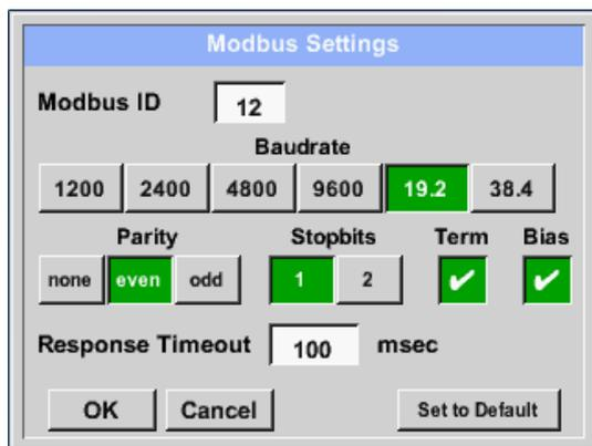
Please insert here the specified *Modbus ID* of the sensor, allowed values are *1 -247*, (e.g. here *Modbus ID = 12*)
