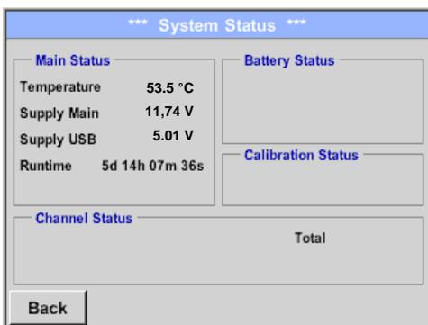
The menu item **“System status”** provides information about the power supply voltages and an operating hour counter.
