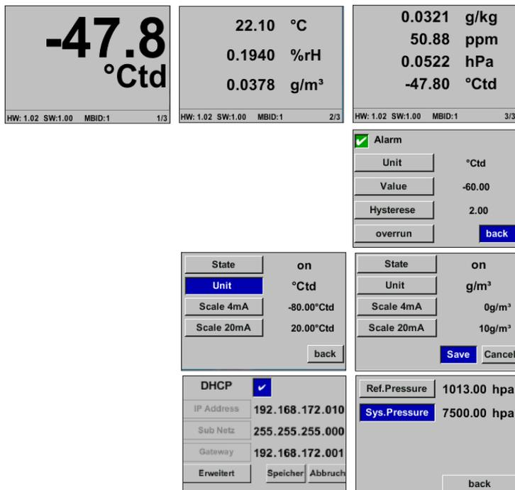
The integrated display shows the dew point in big figures as well as further humidity parameters on two more display pages. The arrow key can be used to scroll between the display pages.
